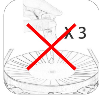
Using more than 3 drops of maintenance oil on the product base at one time is prohibited.
