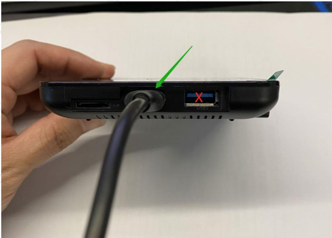
9, There is a reset button in the AV socket of KAT Nexus, use a toothpick or pin to insert the AV port and keep pressing it, Make sure you hear a click, then plug the USB cable into the computer without releasing the Reset button
