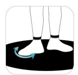
Swiftly turn one foot on the heel at 90 degree and back to normal position to trigger strafing in the corresponding direction. When a stop is needed, take a step.
