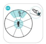
To trigger continuous movement forward without walking, place one of your feet at the center of the platform and keep the other one at its front edge with toes up.
